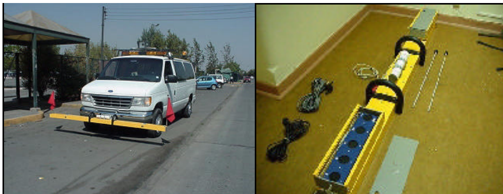
FIGURA 5. TPL, TRANSVERSE PROFILE LOGGER
